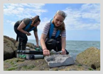
As part of the project, Ecostructure scientists believe they have found a way of attracting marine wildlife to man-made shores. By using photogrammetry and 3D printers to produce moulds, they have created tiles that provide the "nooks and crannies" normally found on natural rocky reef habitat on a coastal defence structure in Borth, Wales.
